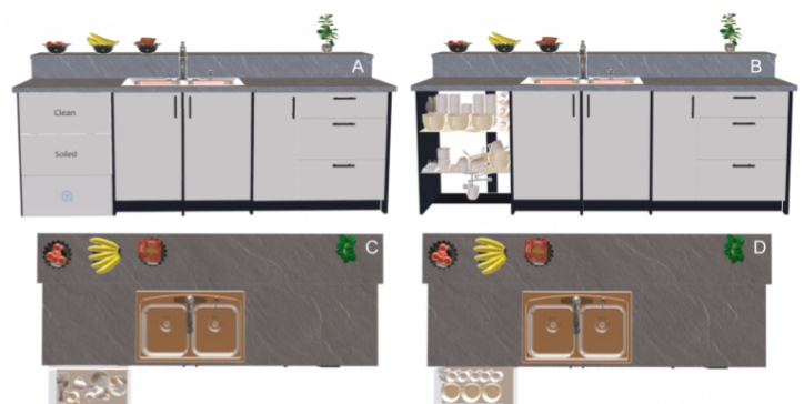
Figure B.1: Dishcare is an autonomous dishwasher. A) Dishcare has a soiled cabinet (middle) where soiled dishes are dropped and a wash module (bottom) where dishes are cleaned and sanitized. Dishcare also has a clean cabinet (top) where clean dishes are organized. A robot located behind the cabinets picks dishes individually from the soiled cabinet, cleans and sanitizes them in the wash module, and organizes them in the clean cabinet; B) Dishcare with front panels removed; C) Dishcare with soiled cabinet open for dropping dishes; D) Dishcare with clean cabinet open for picking clean dishes.
