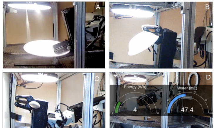
Figure B.3: Dishcare prototype cleans a variety of dish types and conserves energy and water. A) plate cleaning; B) bowl cleaning; C) spoon cleaning; D) Dishcare's energy and water sensors measuring resource consumption while cleaning a mug. Dishcare's robot arm also picks up cups, forks, knives and chopsticks.
